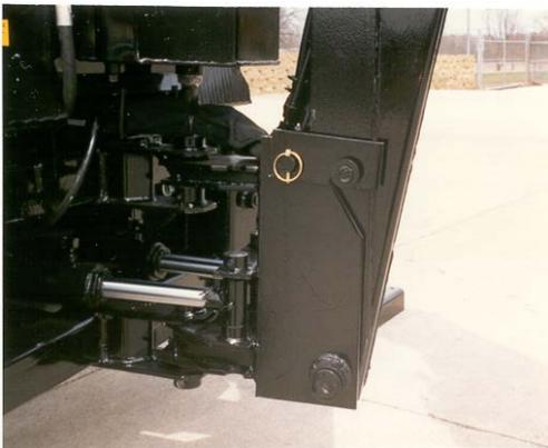
Raise the boom to take the tension off of the transport safety locking bar shown in Figure 14
